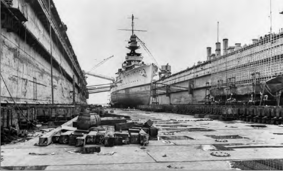
A British warship undergoes a refit in the massive floating dock at Singapore Naval Base. (AWM 007748)
